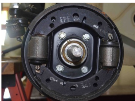
Brake drum and hub have been removed. (The inner bearing stayed on the swivel axle.)
